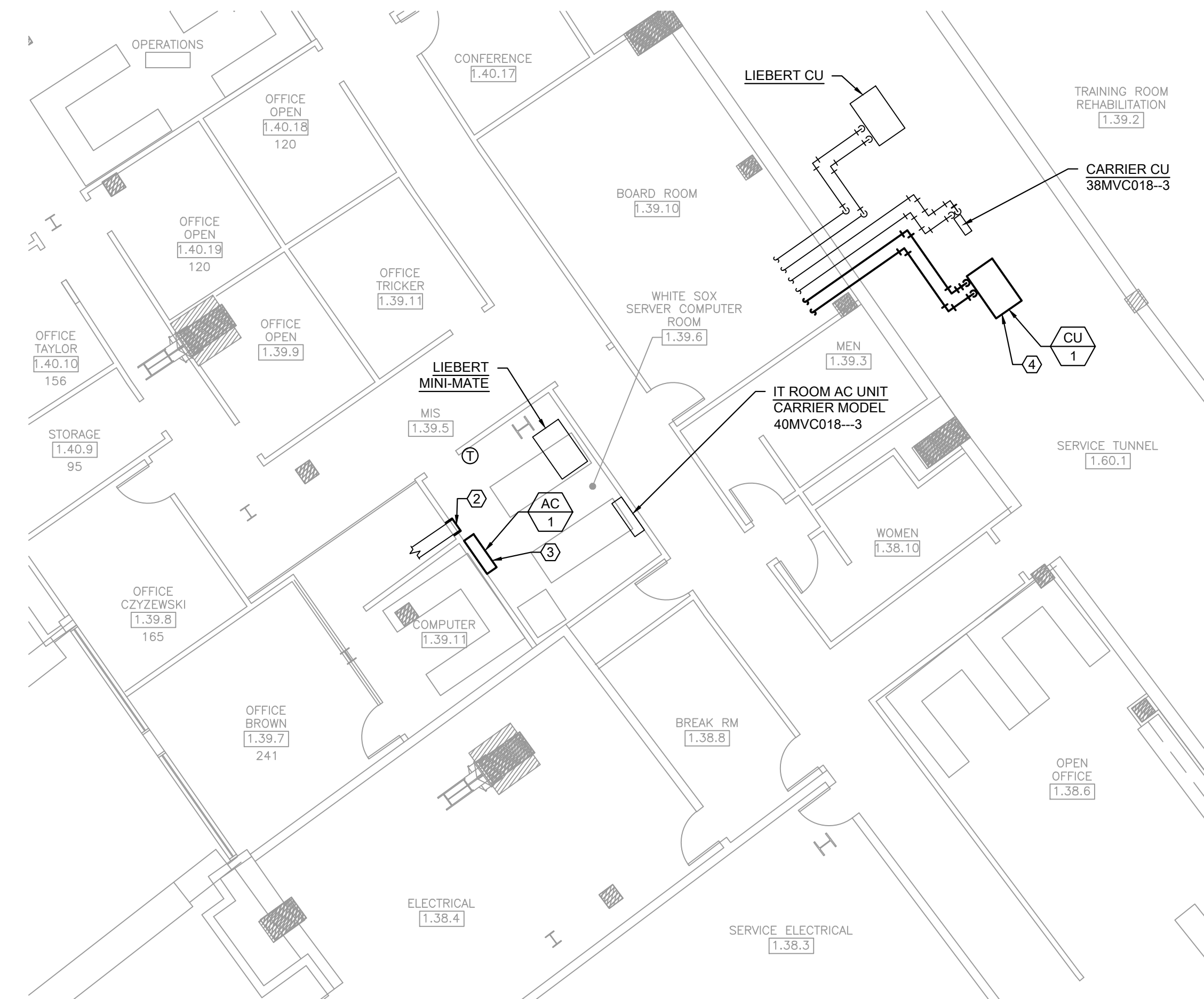
2 MECHANICAL NEW WORK PLAN - IT ROOM SCALE: 1/8" = 1'-0"
